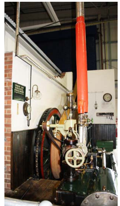
This is the Horizontal Beam Engine, the drive belt is the long strip that wraps around the wheel.
